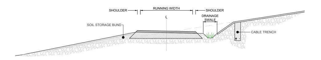
TYPICAL CROSS-SLOPE CUT TRACK SECTION
