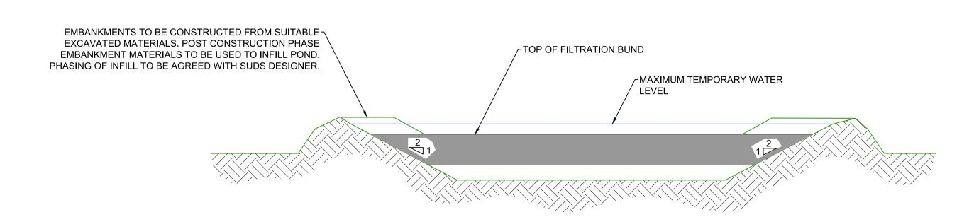
TYPICAL SETTLEMENT POND DETAIL - CROSS SECTION
