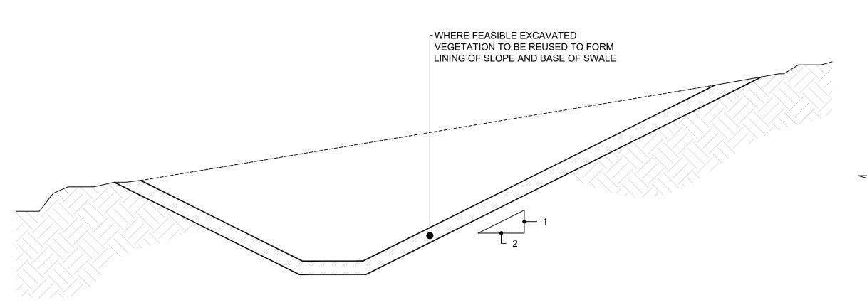
TYPICAL SWALE - CROSS SECTION SCALE - 1:20
